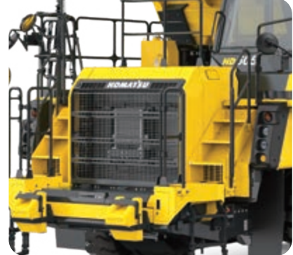
Safe cab access thanks to the low angle of the front stairways with handrails, slip-resistant
